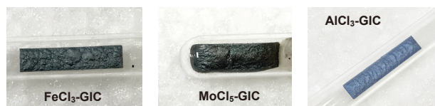
Fig.5 Images of stage 1 FeCl_3 -, MoCl_5 -, and AlCl_3 -GICs.
