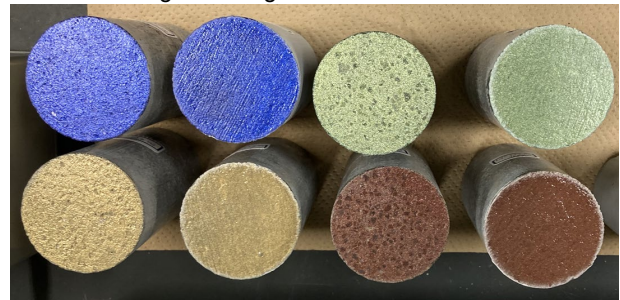
Figure 1. Photographs of the concrete surfaces applying various Chromashine®, type A: left specimen, type B: right one, in the same color.
