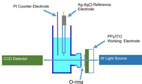
Fig. 1 Schematic diagram of the transparent glass cell.
