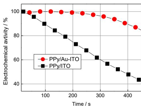
**Fig. 3 Electrochemical stabilities of the PPy films on the Au-ITO or ITO electrodes for applied potential cycles.**
