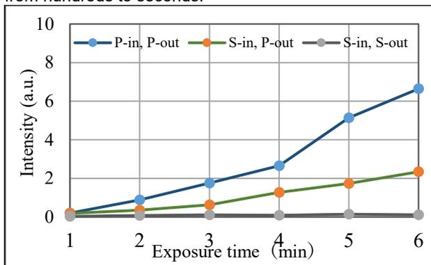
Fig. 3 Reconstruction image intensity at different polarization condition
