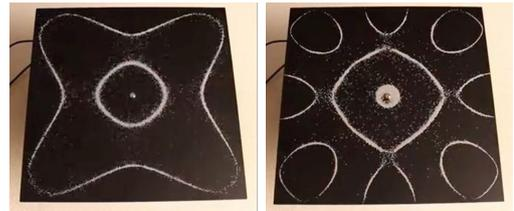
Figure 4. Chladni figures in the various frequencies [1].
