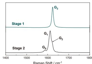
Fig.6 Raman spectra of stage 1 and 2  $MoCl_5$ -GICs.
