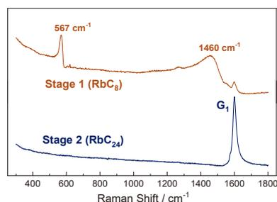
Fig.4 Raman spectra of stage 1 and 2 Rb-GICs.
