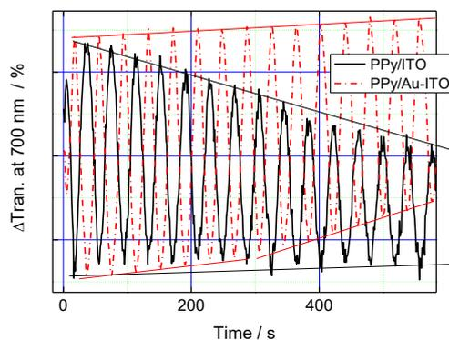
**Fig. 4 Electrochromic stabilities of the PPy films on the Au-ITO or ITO electrodes for applied potential cycles.**
