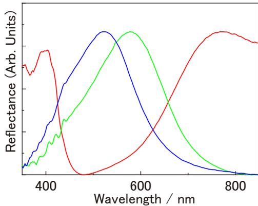
Fig. 2 Typical reflectance spectra of the SCP-urethane paint applying on the concrete surface.
