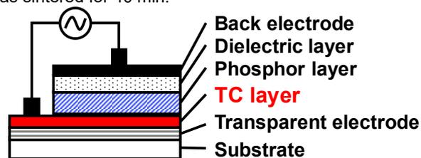
Fig. 1 Structure of powder EL devices
