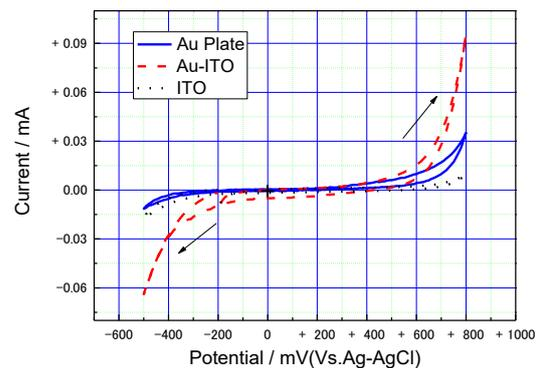
Fig. 2 Cyclic voltammograms (scan rate : 50 mV/s) of the pyrrole polymerization on ITO, Au-ITO and Au plate electrodes at the first potential scanning.
