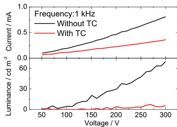
**Fig. 3** Current (top) and luminescence (bottom) dependence of the voltage in powder EL devices with/without TC layer
