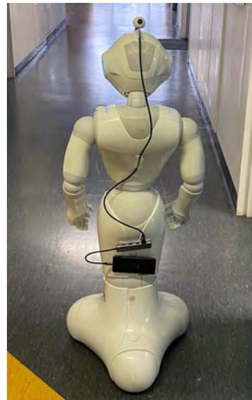
Fig. 1 Pepper robot with 360-degree camera.
