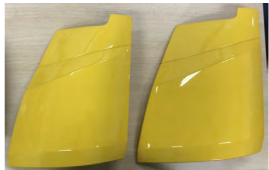
Fig. 3 Appearance of good(left) and defective(right) products by color difference
