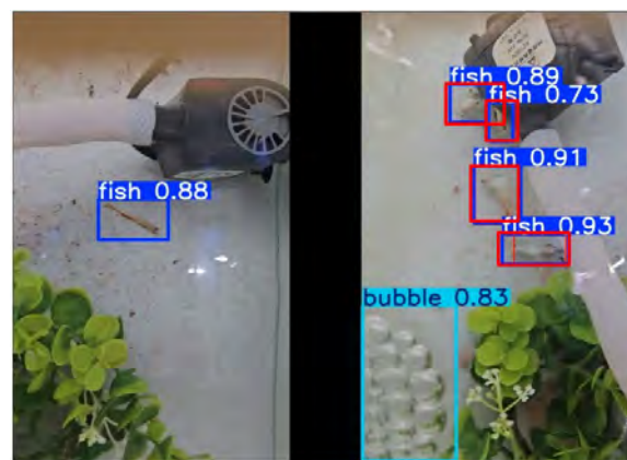
Fig. 3 An example result of detection of dead fish (red rectangles).
