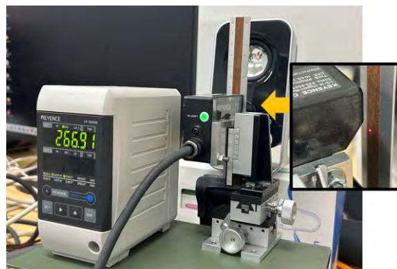
Fig. 4 Setup for detecting the resonance of objects (a rule made of metal here).
