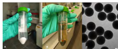
Fig. 2 A) Silica particles before coating; B) Silica particles after coating with PDA; C) Visualization of the silica-PDA particles under TEM microscope ( \approx 180 nm).
