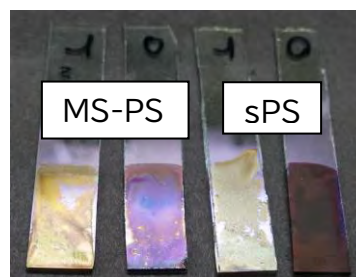
Fig. 3 Photographs of the obtained PMOT film in the reduced state (r) and the oxidative state (o) prepared by MS-PS polymerization and sPS polymerization.
